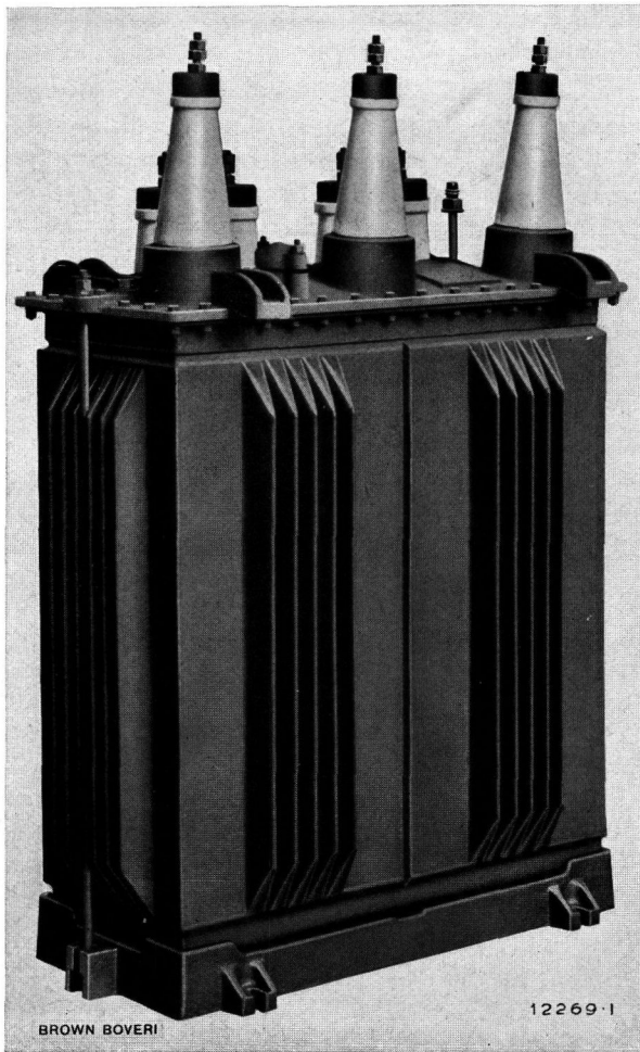
Fig. 3. — Three-phase oil-immersed transformer, Type T 20. 20 kVA, 10000/380 V, 50 cycles.
