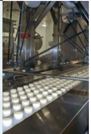
At Ilchester Cheese, an IRB 340 picks the cheese with the help of a vision system that allows it to move at lightning speed.
