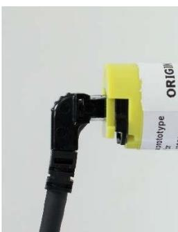
4. Insert the end of the AVT system cable with the right-angle connector in the back of the yellow indicator module. Press firmly into the opening until you feel it latch. Pull back on the connector to verify that it has properly latched. Verify the black tabs on either side are engaged to lock in the cable.
