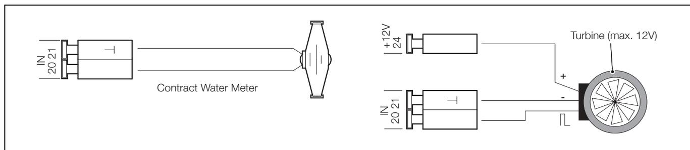
Fig. 4.2 Installation Example for the Water Meter
