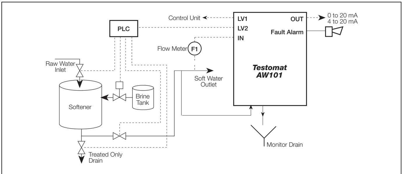
Fig. 3.1 Installation Diagram
