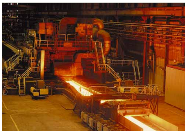
5 Hot-rolling mill in a steel plant. Slabs coming from the melt shop are being rolled into coils.
