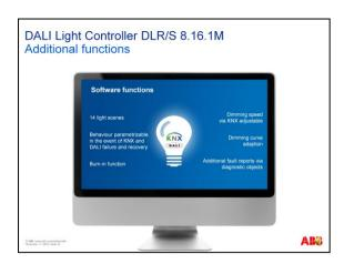
The DALI Light Controller software offers a wide range of functions, such as 14 light scenes, arranged at random from the connected light groups.
