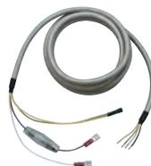
The Cable Set Basic KS/K 4.1 with integrated temperature sensor is used for the connection of a sealed lead acid battery SAK7 to the Uninterruptible Power Supply SU/S 30.640.1 or the Uninterruptible Power Supply NTU/S 12.2000.1.
