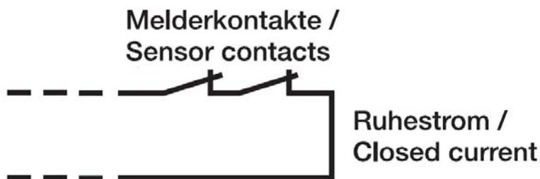
The closed circuit type is closed in its normal state. Should at least one contact open, the circuit is interrupted and it is evaluated by the Security Terminal.
