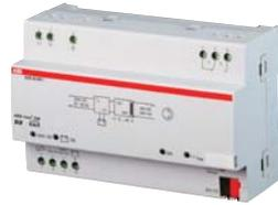
The Uninterruptible EIB / KNX Power Supply SU/S 30.640.1 generates and monitors the KNX system voltage. The bus line is decoupled from the power supply with the integrated choke.
