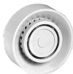
The Electronic Solid-State Siren SSS is used for issuing acoustic alarms within the protected area. An intermittent signal of 2.7 kHz is produced by an electronic tone generator and converted into sound waves by a piezo element.
