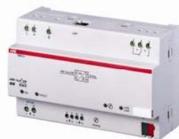
Using the Telephone Gateway TG/S 3.2, it is possible to send configurable voice messages via the telephone network. As well as voice messages, emails or SMS messages can be sent. If the device is called, it is possible to navigate through a menu using dial tones (DTMF), where states can be queried and commands can be executed.
