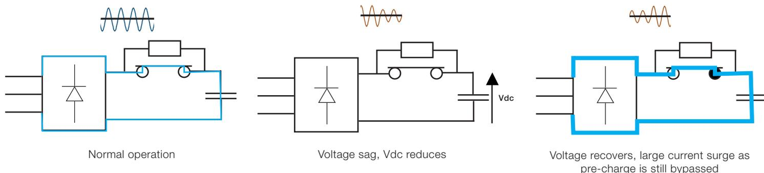
Figure one: **Top** normal controlled startup process. **Bottom** Inrush currents following a voltage sag
