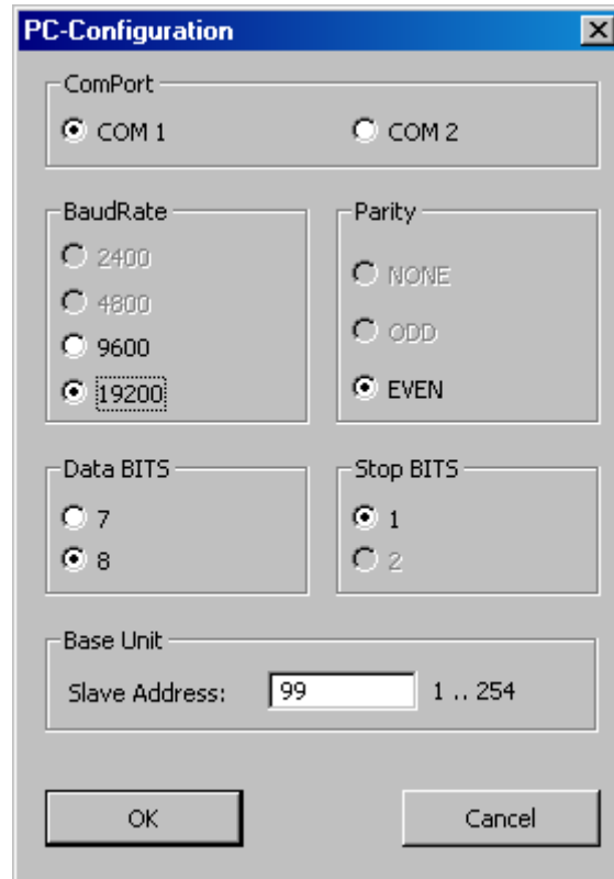
Figure 30: Operating Tool: setting the communication parameter of the serial port.
