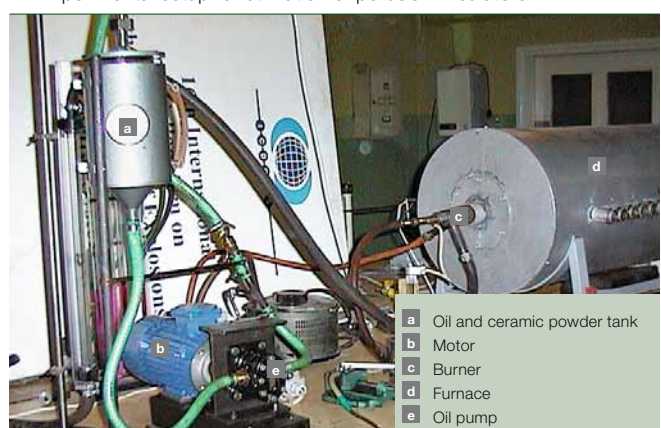
6 Experimental setup for utilization of porcelain insulators
