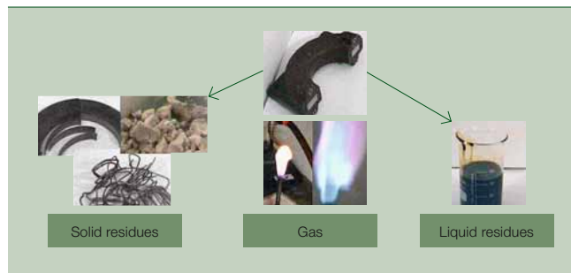
2 Products from pyrolysis of used epoxy product
