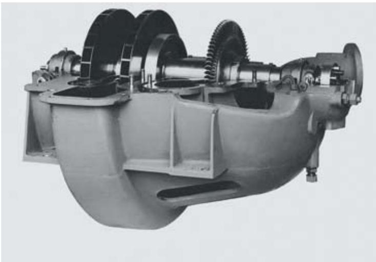
World's first turbocharger for a large diesel engine. Delivered in 1924, it had external plain bearings and a two-stage compressor for a pressure ratio of 1.35.
