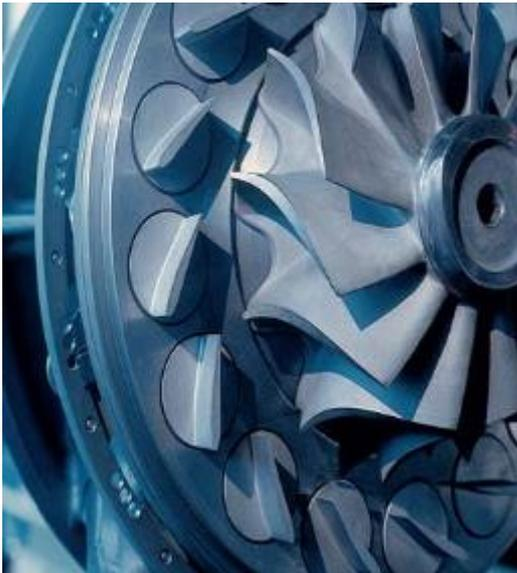
Variable nozzle ring of a TPS57 VTG turbocharger
