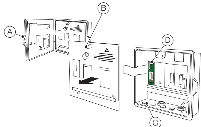
**Figure 5 Ethernet connection**
