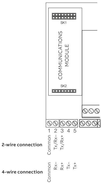
**Figure 3** 2-wire and 4-wire Modbus serial links
