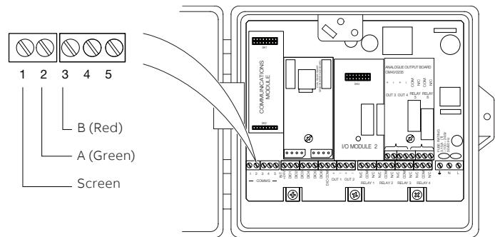
**Figure 2** Aztec AWT440 PCB connections to PROFIBUS network
