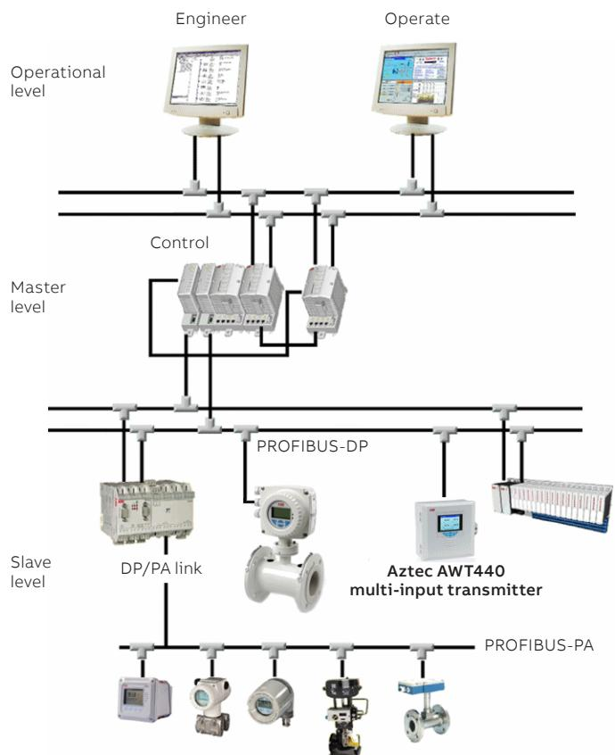
**Figure 1 Typical PROFIBUS network**
