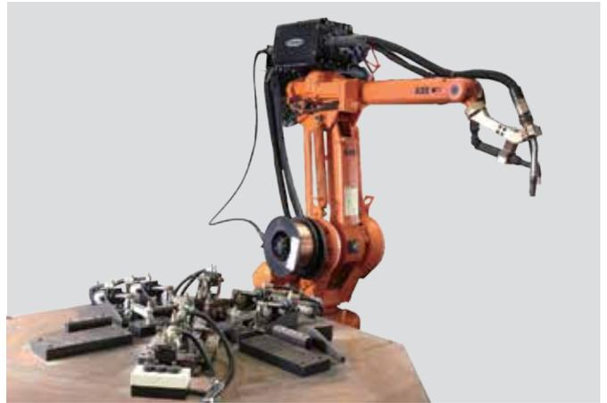
Welding robot, to ensure stable and reliable welding quality
