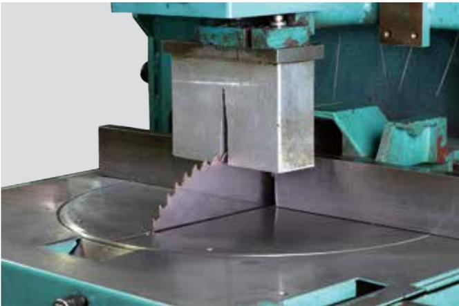
Circular sawing machines made in Germany ensure the flat faying surface of the busbar. Advanced cutting and plating process brings the smoothness of conductor section
