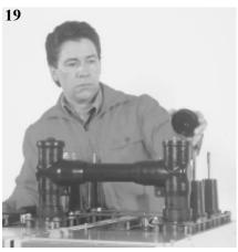
5. Fix covering cap to the adapter casing (Photo 19)
