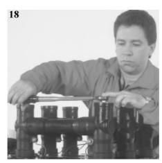
4. Clean adapter and insulating plug (area "D") and coat with assembling paste. Push insulating plug (key size 19) together with a clean cable tie (see page 4 no. photo 13) (to ventilate) into the adapter and screw lightly together.
