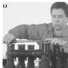
3. Clean adapter and bushing (area "B") and coat with assembling paste. Slide the adapter onto the bushing. Screw together threaded bolt with tightening washer and nut, torque 50 Nm.(Photoes 8-13)
