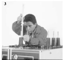
1. Screw threaded bolt manually into the bushing until stop. Then tighten to 10Nm torque. The threaded bolt must project from the bushing 79±2mm. (Photoes 1-3)
