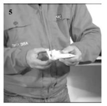
Clean contact shells and adapter (area "A") and coat with assembling paste.
