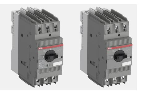
ABB's MS165 manual motor starters and MO165 manual motor starters magnetic only, are electromechanical protection devices for the main circuit. They are mainly used to provide fuseless protection of motors against short-circuits, overloads and phase failures. In addition, they are used to switch motors ON/OFF manually. Starter combinations are setup together with contactors.
