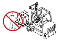
• Do not stand near the EVSE during handling
