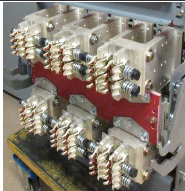
Figure 10A. AKD-8—(3200-5000A) Primary Contacts or “Fingers” (Apply Grease)
