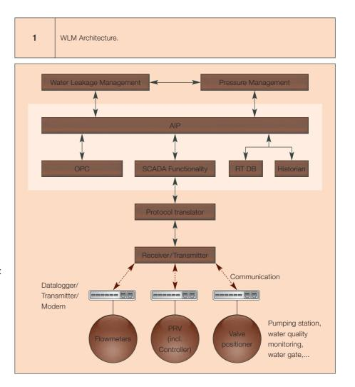
Advise<sup>IT</sup> Water Leakage Management To address this concern, ABB started its "Water Leakage Management" project. The goal is to help water and water management companies reduce and manage the loss of water from their system in the form of bursts and background leakage. *AdviseIT Water Leakage Management (WLM)* was born out of this concept. It is developed based on ABB's Industrial IT platform **1**.
