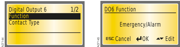
Figure 7.28 Digital Output 6 - Function, Emergency/Alarm is the default
