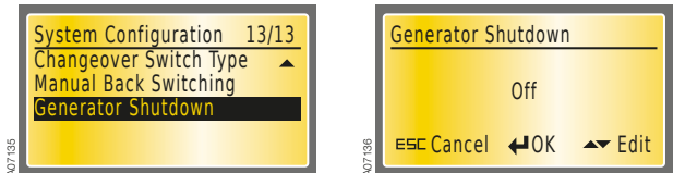
Figure 7.22 Generator Shutdown, Off is the default
