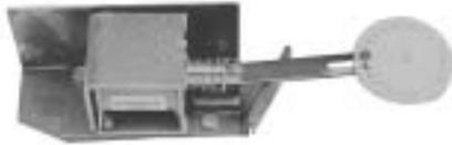
Shunt Trip operation is available for local push button or remote trip applications. This device utilizes a solenoid to actuate the "A" or "KS" mechanism trip latch. The Shunt Trip is available in a complete range of AC and DC control voltages. Use of the shunt trip requires an auxiliary switch (below) to assure momentary actuation of the shunt trip coil.
