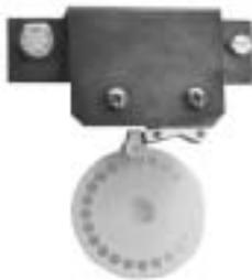
An optional Fuse Auxiliary Switch is available to indicate an open fuse condition. This switch has two contacts, one normally open and one normally closed, and is actuated by the tie rod linkage connected to the fuse base.
