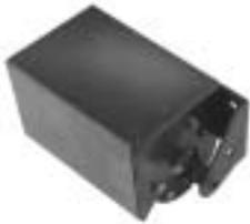
The optional Auxiliary Switch is available with six or eight contacts, configured with an even number of normally open and normally closed contacts. The Auxiliary Switch is mounted to the chassis and changes state when the VersaRupter or grounding switch is opened or closed.
