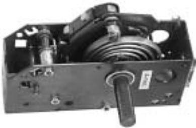
The A-Mechanism is a dual spring, stored energy device that is well-suited for remote tripping applications. The opening spring is charged and latched by an operating handle (direct or chain drive), or by a motor operator. The switch is then opened by any of several methods:
