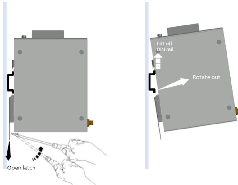
Figure 6: Removing AWIN GW100 rev.2 from the DIN rail
