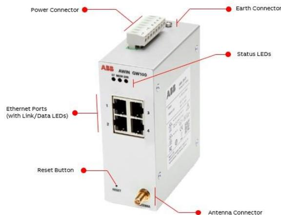
**Figure 1: AWIN GW100 rev.2 gateway and its interfaces**
