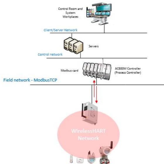
Figure 35: AWIN GW100 rev.2 connectivity to control system (AC800M)
