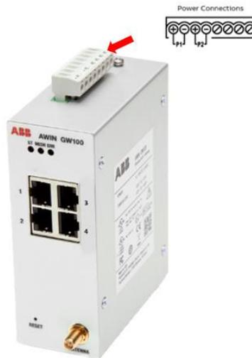
**Figure 7: AWIN GW100 rev.2 power connections**
