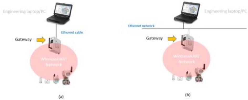
Figure 34: AWIN GW100 rev.2 configuration via (a) direct connection, or (b) network to a PC
