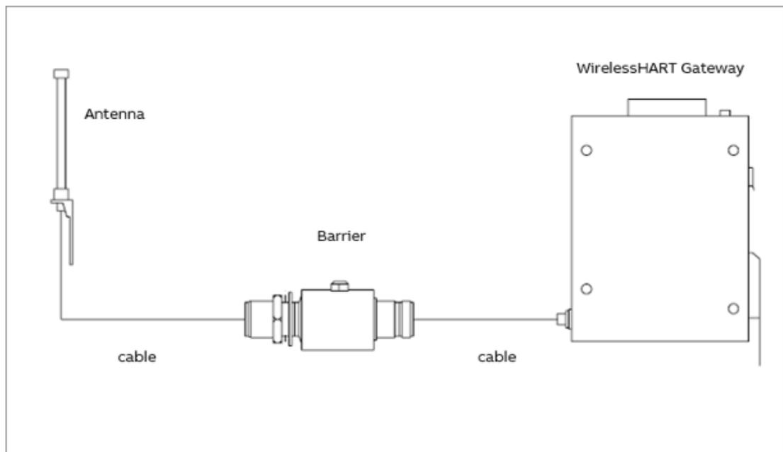
**Figure 33: Example of remote antenna assembly**
