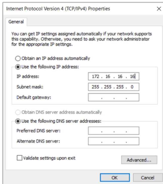
Figure 8: Properties window to change IP address of a PC
