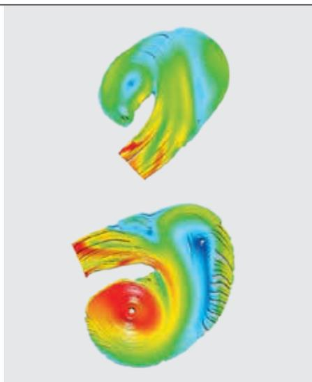
8b Undesired flow separation and recirculation in diffuser
