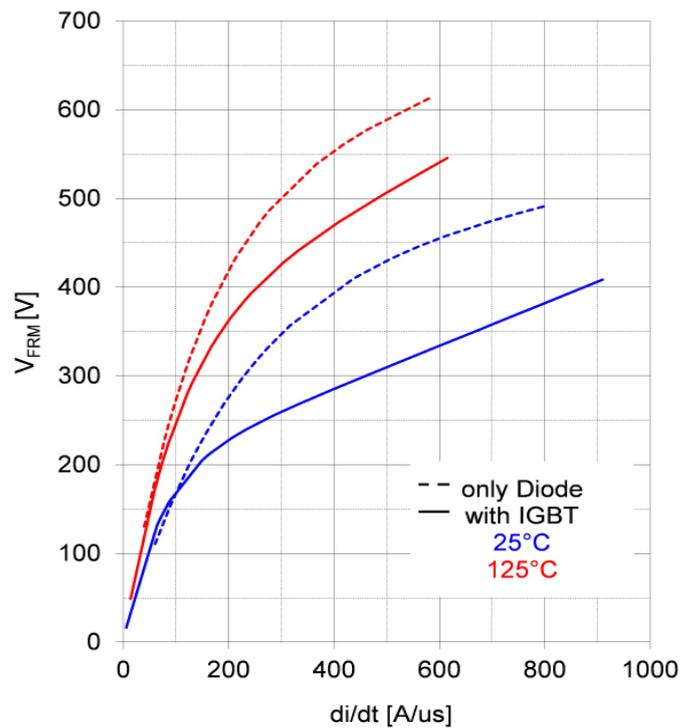
Figure 6 Forward voltage di/dt dependence, with and without antiparallel IGBT
