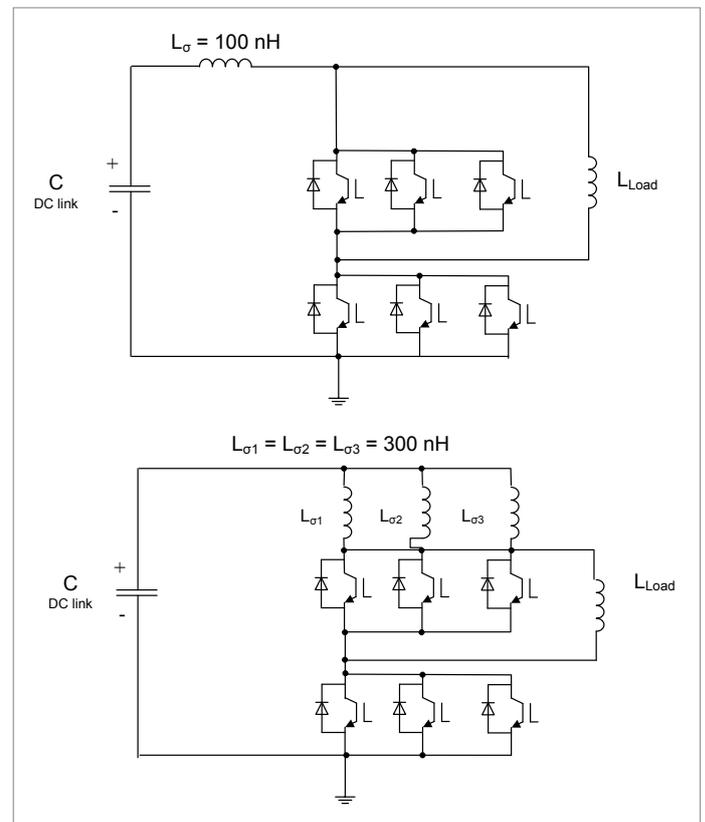
Figure 4 Inductances at different configurations to achieve the same di/dt.
