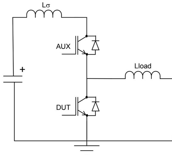
Figure 1 Test circuit for the dynamic performance of the diode
