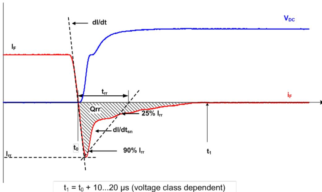
Figure 2 Definitions for the diode turn-off parameters
