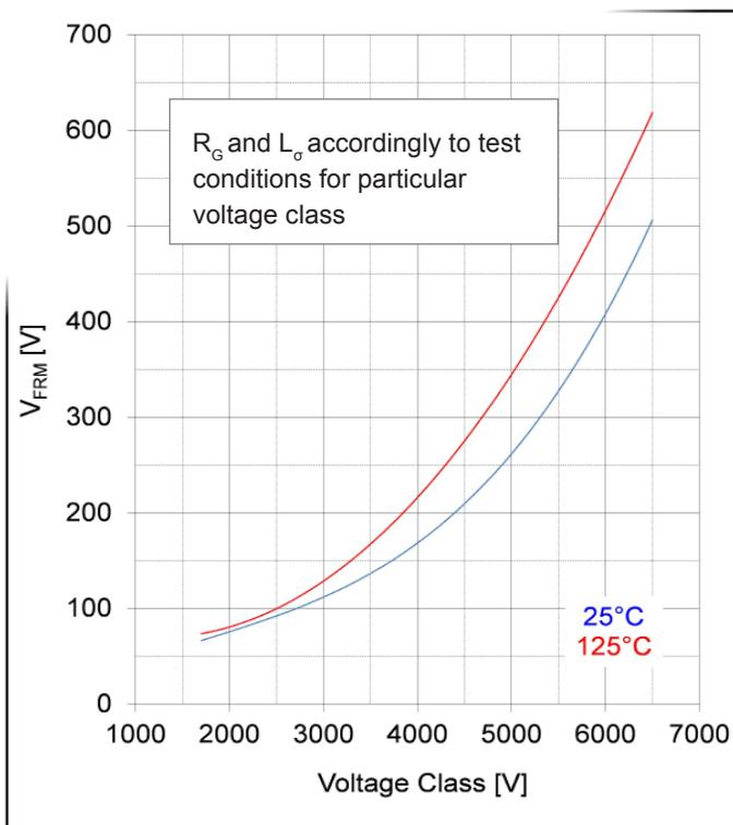
Figure 5 Forward voltage dependence of blocking voltage.
