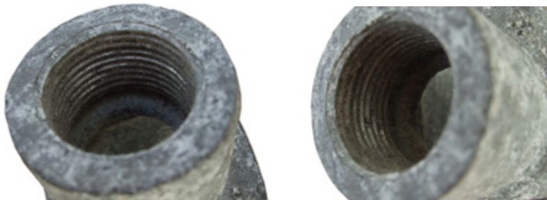
The T&B Fittings conduit bodies display clean threads with only salt deposits.
