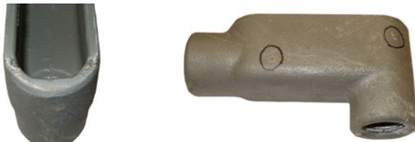
Competitor 2 conduit bodies show signs of pitting and paint flaking.
