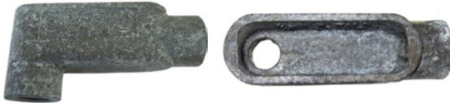
The T&B Fittings conduit bodies are free of any pitting inside and out—only salt deposits.
