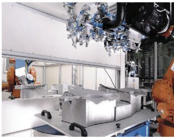
Developed by Robot Technology GmbH The laser robot is based on an ABB IRB 4400 robot. The CO2 (obs se till att 2 blir nedsänkt) laser has an inherently stable laser housing with axes 4 and 5, which replace the standard main axes of the robot.
