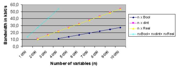
*Figure 12. Required bandwidth on Control Network to get 10sec update rate of AC 800M OPC server*
