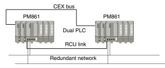
Figure 5. Example of a redundant CPU configuration.
