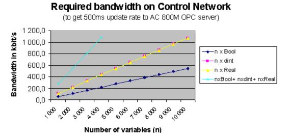
*Figure 11. Required bandwidth on Control Network to get 500ms update rate of AC 800M OPC server*
