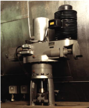
Figure 34: Linear actuator (feed-water preheating)
