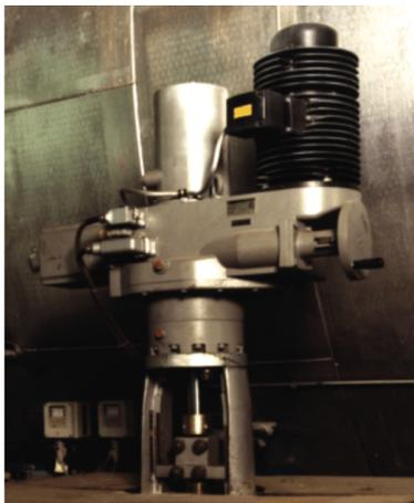
Figure 34: Linear actuator (feed-water preheating)
