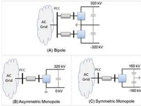
**Figure 4: Configurations of VSC HVDC converter stations**
