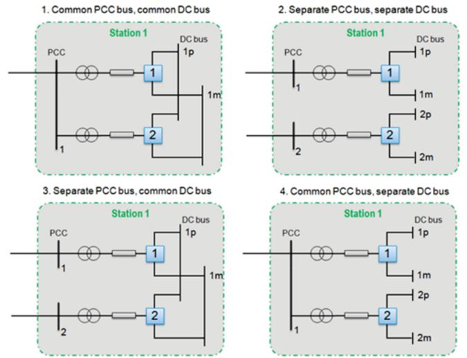
**Figure 6: Configurations for two parallel monopole converters in a station**
