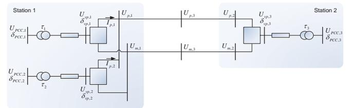
**Figure 7: Two terminal monopole grid with a converter-less bus**
