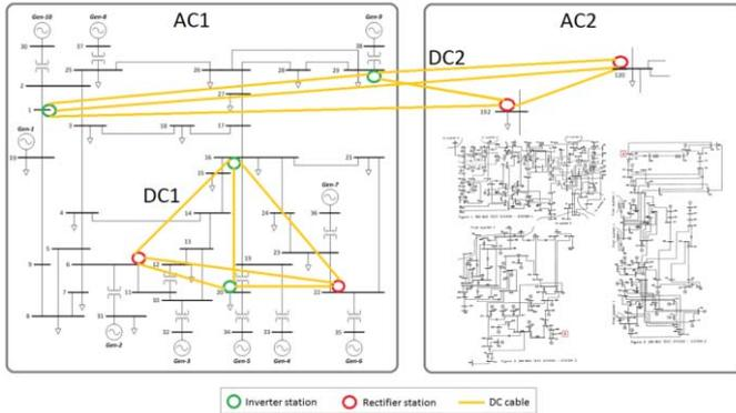
**Figure 1: Hybrid AC/HVDC grid example showing two interconnected AC grids and DC grids**
