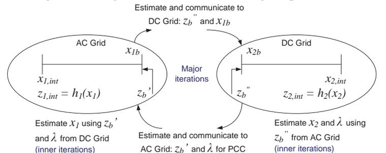
**Figure 3: Data exchange across the boundaries during the iterations**
