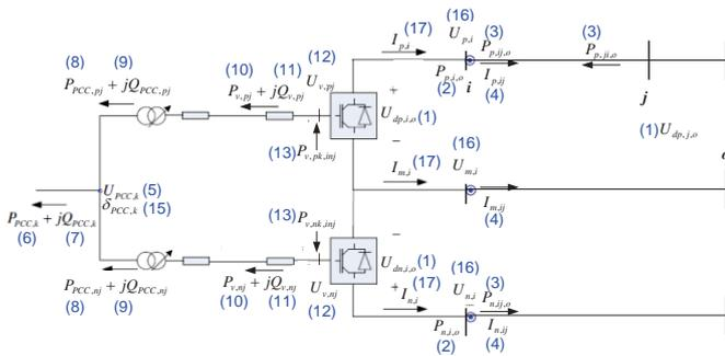
**Figure 5: Bipole configuration and the measurement types**
