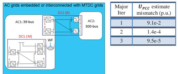
**Figure 12: (left) the test system with monopole (M) and bipole (B) grids, (right) major iterations and PCC state mismatch**
