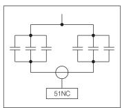
secondary measures the current which circulates over the connection - current which in the absence of a fault is equal to zero (two balanced three-phase banks), whereas it is different from zero in the presence of a fault; the code of the protection is 51NC (unbalance current for capacitor banks);
