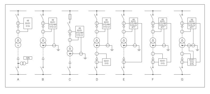
The following figure shows some configurations of the protection system which can be selected according to the power of the machine, the connection unit and the status of the neutral.
