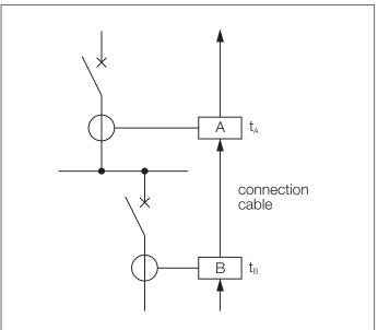
Logical type selectivity allows trip times to be reduced and full selectivity to be obtained in any case. The protections must be interconnected to allow the changeover of locks and consents (by means of pilot conductors and not by means of supervision systems which have incompatible response times) to allow correct operation. If the protections were not interconnected, there would be rapid tripping of all the protections run through by the fault current.
