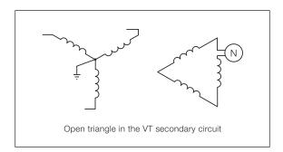
G when the protection is connected directly to the secondary of a transducer (CT or VT) which measures the homopolar parameter directly (current or voltage);
