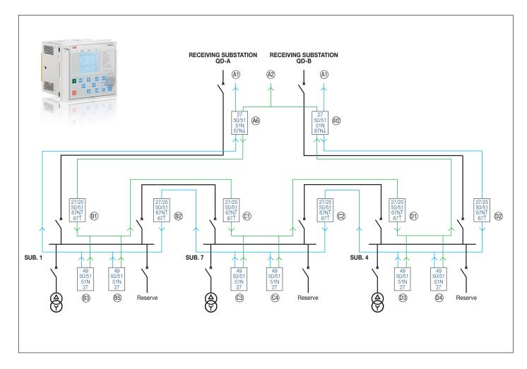
the faulted part, but substations not affected by a fault are not stopped). It is, in any case, obvious that more complex systems can be made where, for example, even more sophisticated logical selectivity can be made (with only the busbar or cable fault out of service) and particular functions activated (important with small-sized transformers as ring networks typically are), such as failed circuit-breaker opening 50BF.
