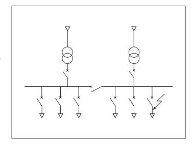
From the theoretical point of view, calculation of the short-circuit currents should be processed using the data obtained from studying the voltage profiles. In reality, the Standards envisage that the calculation be made at the rated plant values and appropriate correction coefficients are introduced for compensation (voltage factor 'c').
