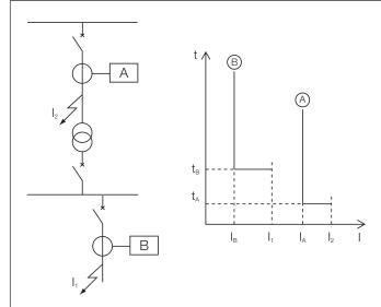
With regard to time graduation, this must take into account the characteristics of the apparatus present in the plant, and in the specific case of the medium voltage networks:
