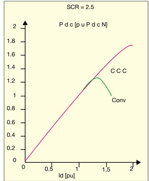
Figure 2. The CCC is in a stable situation, while the conventional converter is close to the stability limit
