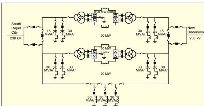
Figure 1. Single line diagram of the Rapid City DC Tie
