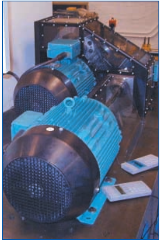
Multidrive involves two motors and drives, with one set motoring and the other generating; this unit is designed for the testing of cambelts
