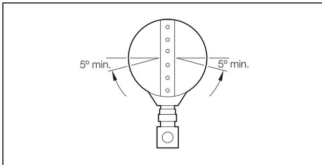
Fig. 2.4 Horizontal Pipe Mounting – Liquids
