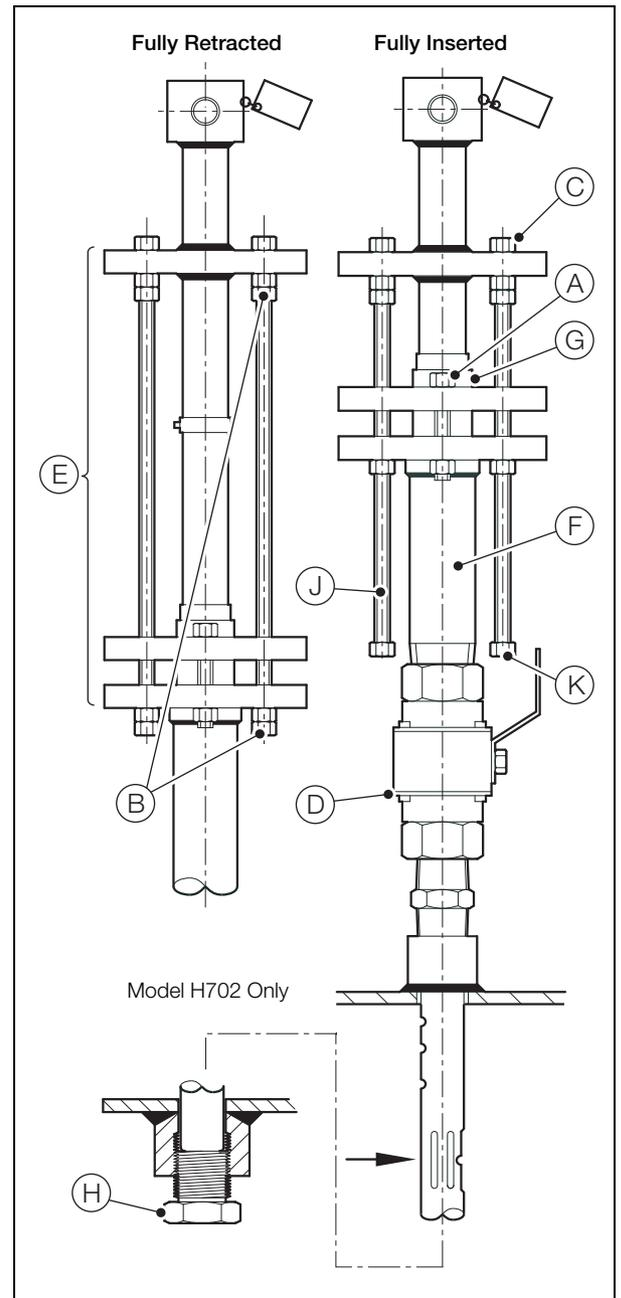
Fig. 3.2 Removing and Refitting Models FPD350.(H6/H7)
