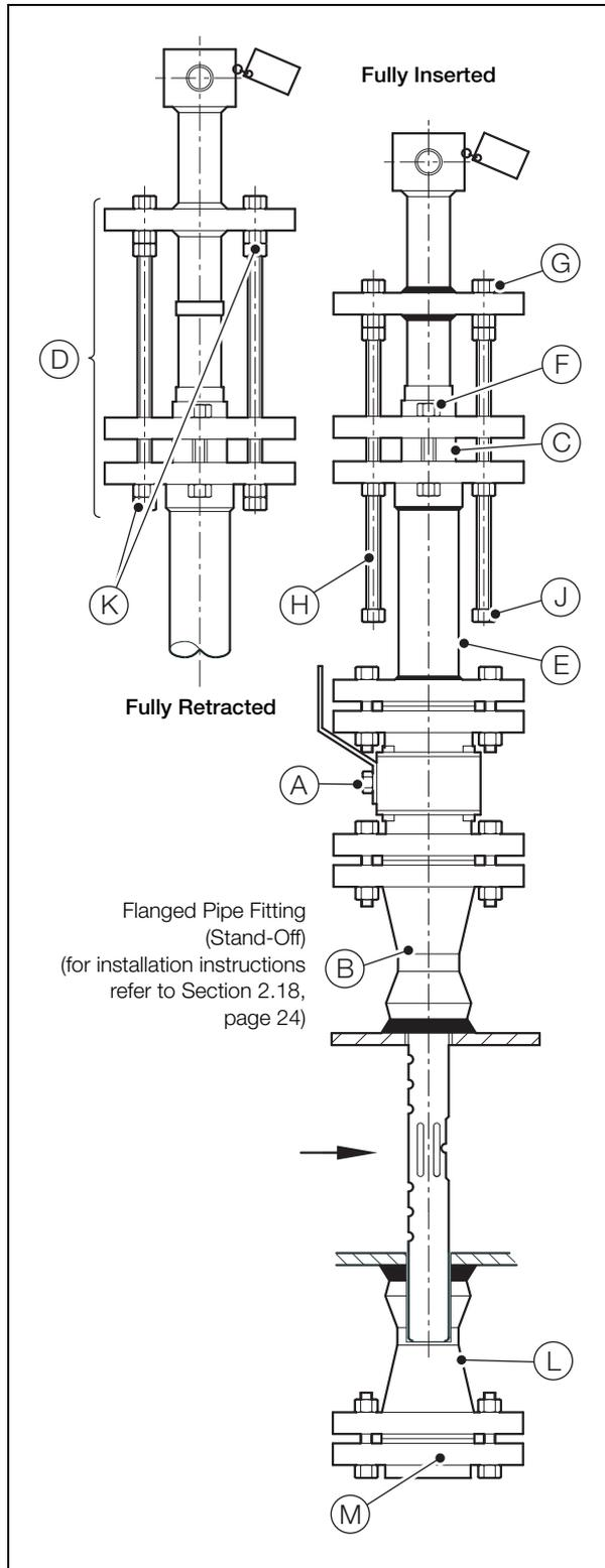
Fig. 2.16 Installation of Flanged Models
