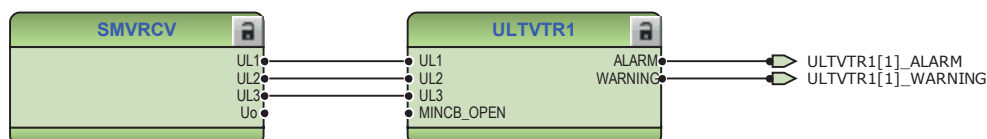
Figure 92: Connection of SMVRCV to ULTVTR1 in Application Configuration
