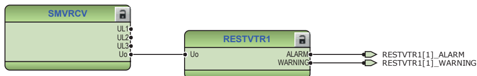
Figure 54: Connection of SMVRCV to RESTVTR1 in Application Configuration
