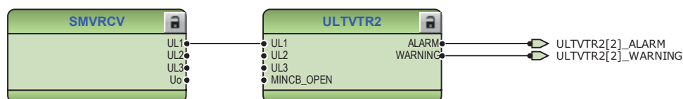
Figure 94: Connection of SMVRCV to ULTVTR2 in Application Configuration
