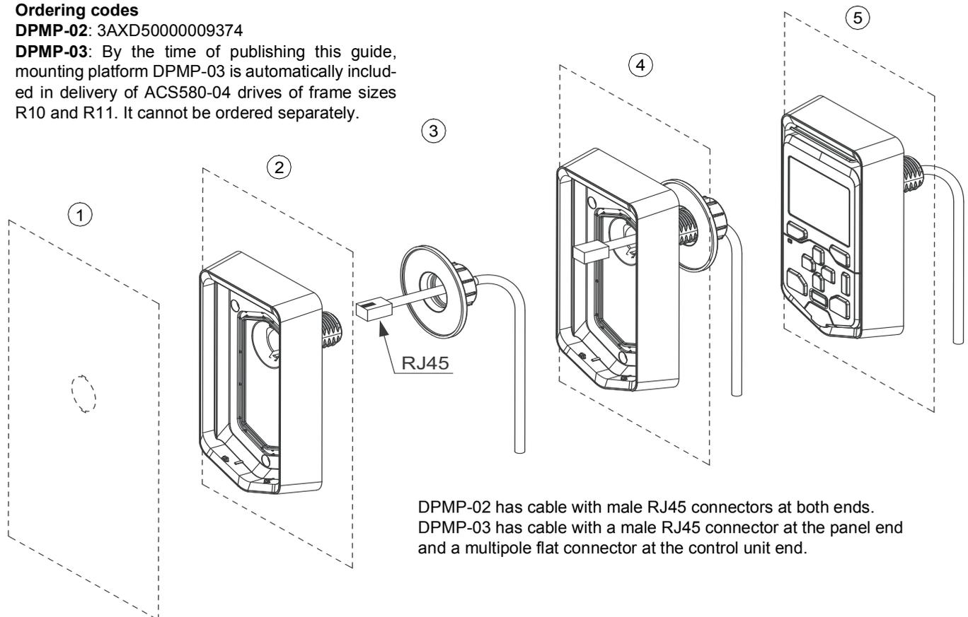
DPMP-02 has cable with male RJ45 connectors at both ends.
