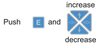
Fig. 4.1.2.4.-1 Adjusting the display contrast
