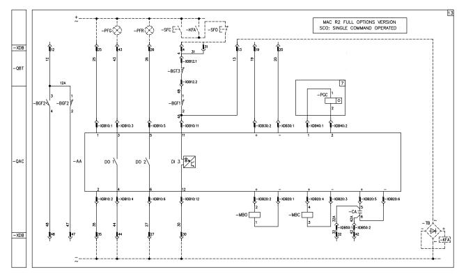
WARNING: the voltage at the feeder clamps of the electronic card and the command circuit (clamps 1-3-5-11 and 2-4-6-12) must come from an unique auxiliary circuit supply and the same circuit breaker.
