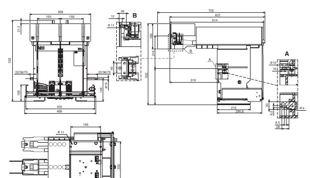
VSC 7/FN Contactor preset for 2 BS fuses in parallel
