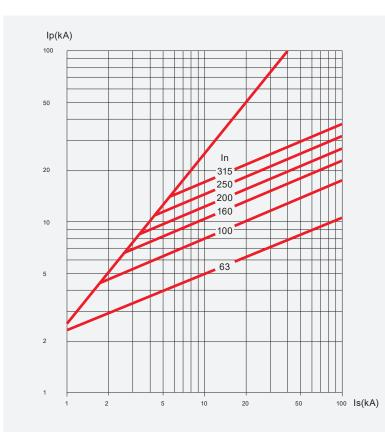
Is = prospective short-circuit symmetrical currentIp = current limited by the fuse (peak value)
