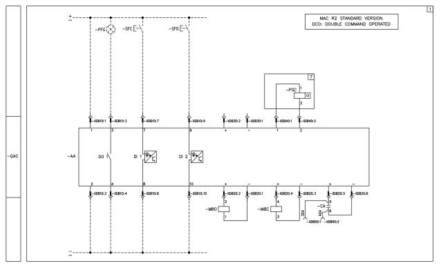
WARNING: the voltage at the feeder clamps of the electronic card and the command circuit (clamps 1-3-7-9, 2-4-8-10 of fig. 1 and clamps 11, 12 of fig. 2) must come from an unique auxiliary circuit supply and the same circuit breaker.
