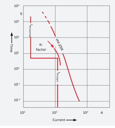
Fig.  $\ensuremath{\mathsf{E}}$  - Motor circuit protection as specified in the relevant standards
