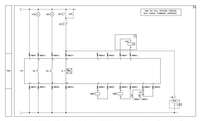
WARNING: the voltage at the feeder clamps of the electronic card and the command circuit (clamps 1-3-5-11 and 2-4-6-12)must come from an unique auxiliary circuit supply and the same circuit breaker.
