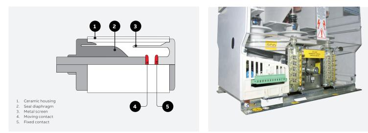
Schematic cross-section of the vacuum interrupter.
