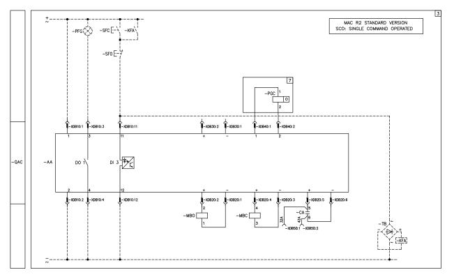
WARNING: the voltage at the feeder clamps of the electronic card and the command circuit (clamps 1-3-11 and 2-4-12) must come from an unique auxiliary circuit supply and the same circuit breaker.
