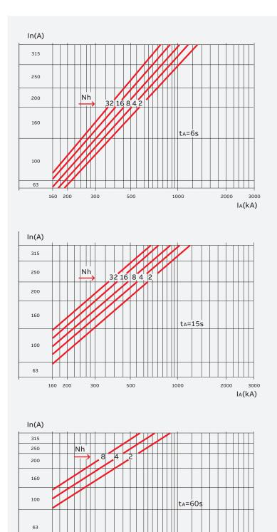
• Rated current In. This must be selected by consulting the diagrams indicated in fig. A which refer to the case of starting at regular time intervals, except for the first two start-ups of each hourly cycle which can take place in immediate succession.
