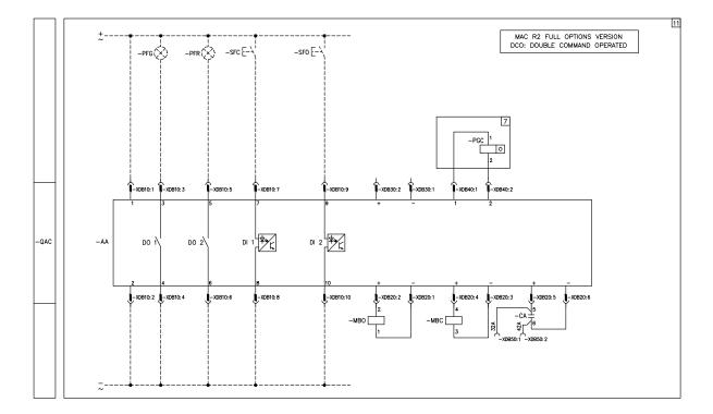
WARNING: the voltage at the feeder clamps of the electronic card and the command circuit (clamps 1-3-7-9, 2-4-8-10 of fig. 11 and clamps 11, 12 of fig. 2) must come from an unique auxiliary circuit supply and the same circuit breaker.
