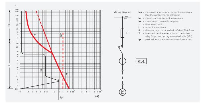
Fig. D - Graph showing the coordination between 250 A ABB CMF fuse and relay with inverse time delay trip.
