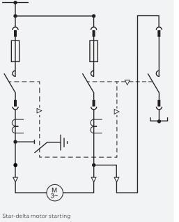
Fig. F - Typical diagrams of transformer power supply and motor starting
