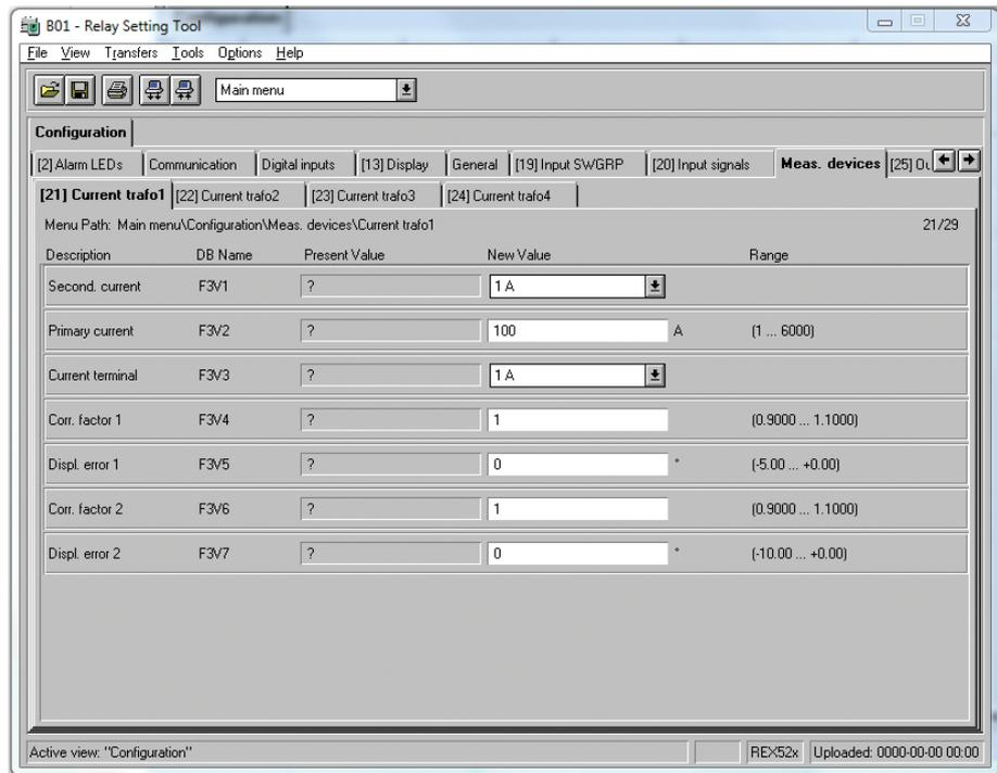
Figure 35: Current transformer ratio parameter setting in REX 521
