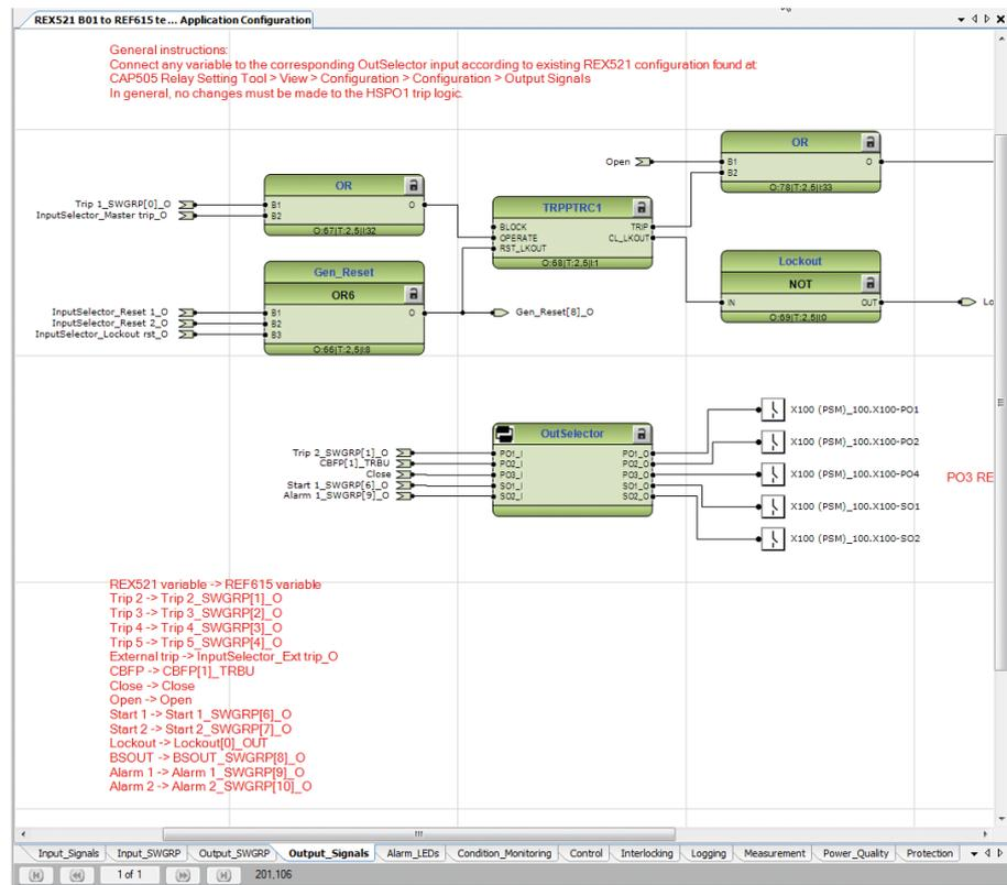
Figure 32: Output signals in the PCM600 configuration template
