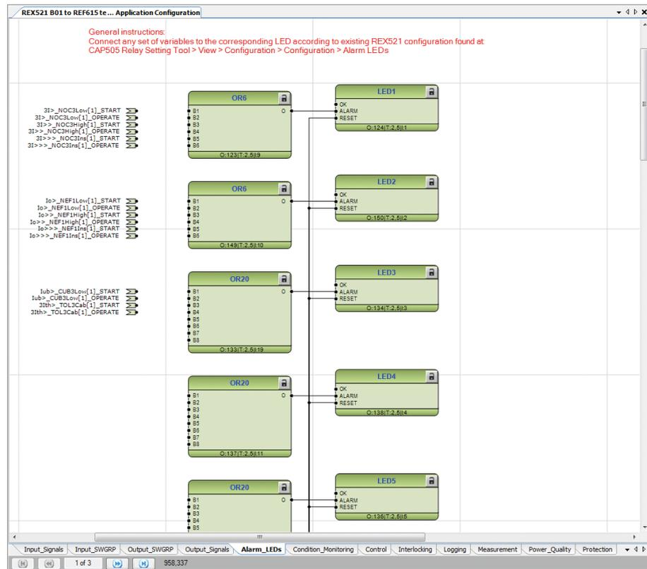
Figure 34: Alarm LEDs in the PCM600 configuration template
