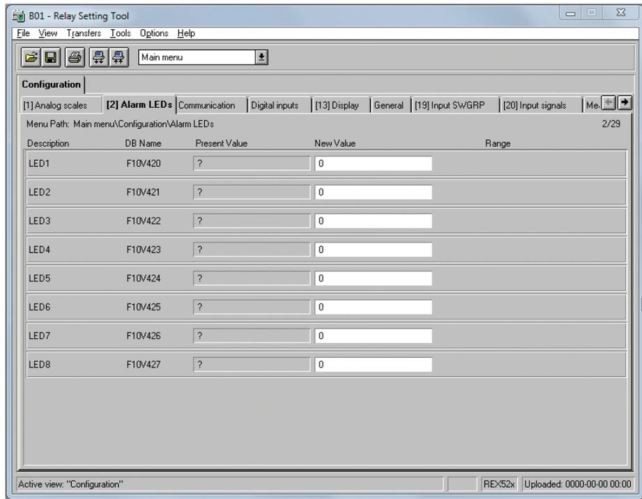
Figure 33: Alarms LEDs in REX 521
