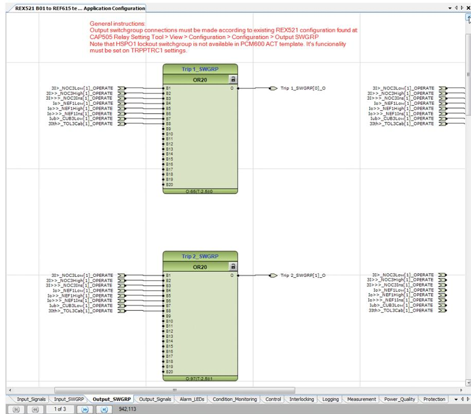
Figure 30: Output switchgroups in the PCM600 configuration template
