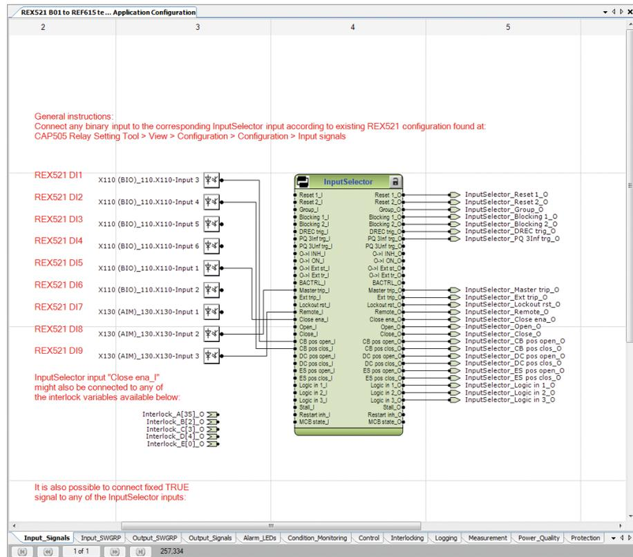
Figure 26: Input signals in the PCM600 configuration template
