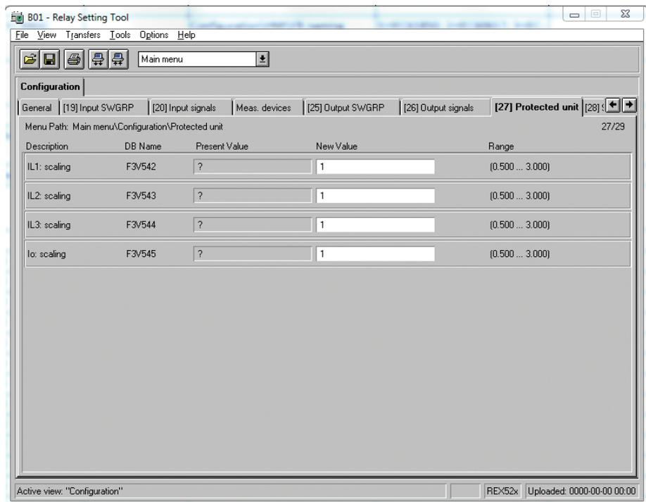
Figure 36: Scaling factor parameter setting of the protected unit in REX 521
