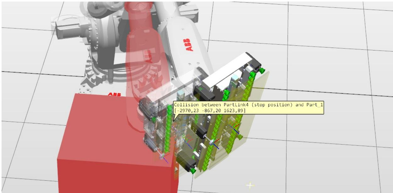
Toggle between nominal and stop position graphics in the Recording Playback window.
