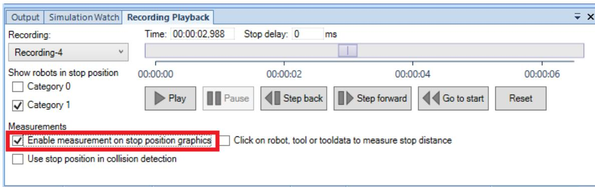
There is also a stop distance measurement mode which lets you measure the distance between a point on the robot at stop position and the corresponding point at the nominal position with one click.
