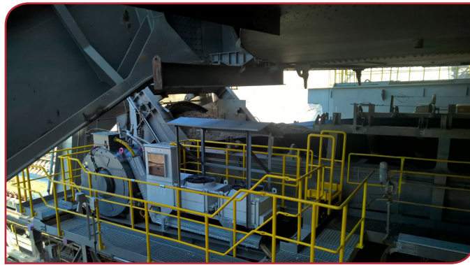
Left: Pilot low voltage GCD installation based on permanent magnet motors.
