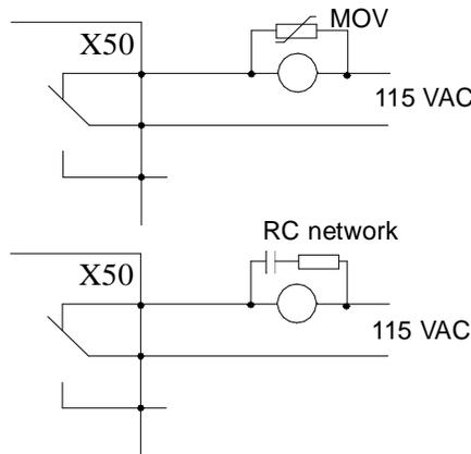
MOV should be rated 120 VAC - 240 VAC for 115 VAC circuits, 240 VAC - 320 VAC for 230 VAC circuits, minimum 10 joules. Values for the RC Network vary, as they effect the opening and closing time. Contact the contactor manufacturer for recommended values.
