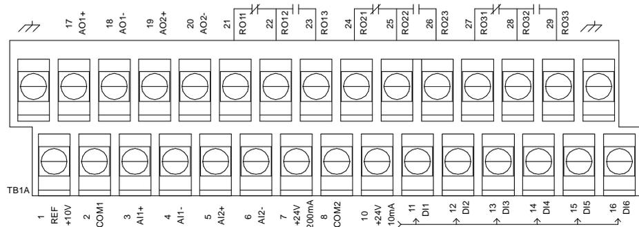
**Potentiometer** A manual speed potentiometer is connected to the reference at TB1:1 (+10 VDC) and TB1:2 (common), and to one of the analog inputs. When the speed potentiometer is supplied from the factory for manual (Hand) operation, it is connected to AI2 (TB1:5).
