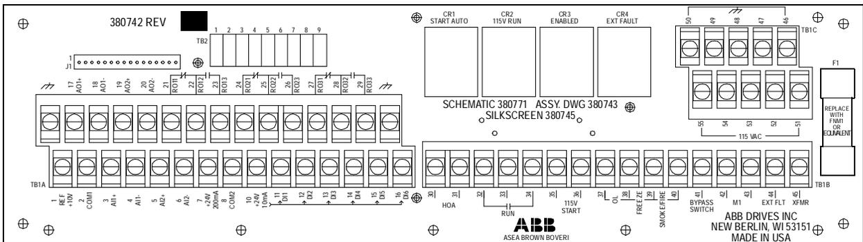
Terminals TB1:1 through TB1:20 are low voltage terminals (24 VDC maximum). Terminals TB1:21 through TB1:29 are relay output terminals. Ground terminals are located next to TB1:17 and TB1:29. These are to be used to connect the shields of shielded cables. Terminals TB1:30 through TB1:55 are 115 VAC control. These terminals are not used when the 115 VAC Control Transformer is not supplied. Connection to all of these terminals is described in the following paragraphs.
