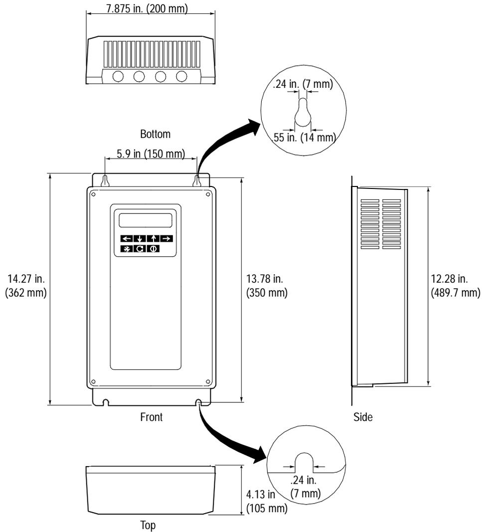
Figure 4-4 Example of Control Box Mounting
