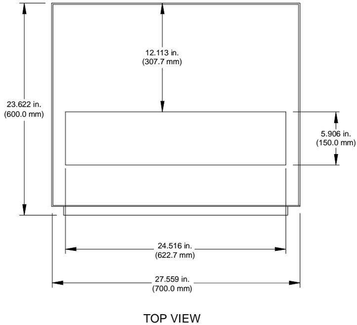
Figure 3-3 ACS 502 Conduit Entry Area for Two Door Enclosure
