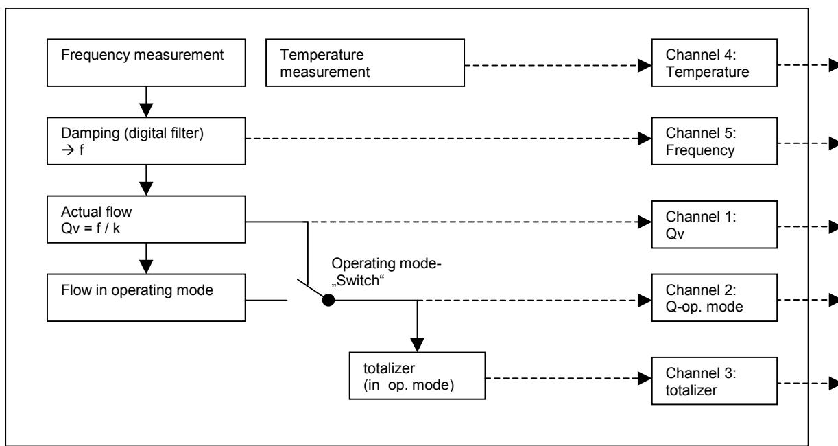
The Primary (Vortex or Swirl flow meter) generates a frequency signal. Using the calibration factors (k-factors) and damping parameter the converter calculates the actual flow value  $Q_v$ . In accordance to the operating mode a flow value is calculated (e.g. mass flow( $Q_m$ ), normal flow ( $Q_N$ )) and is the input for the flow totalizer. Additionally the temperature of the flow medium is measured, if this option is selected by ordering the device.
