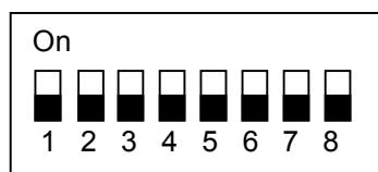
Switch 1 = Simulate Enable
