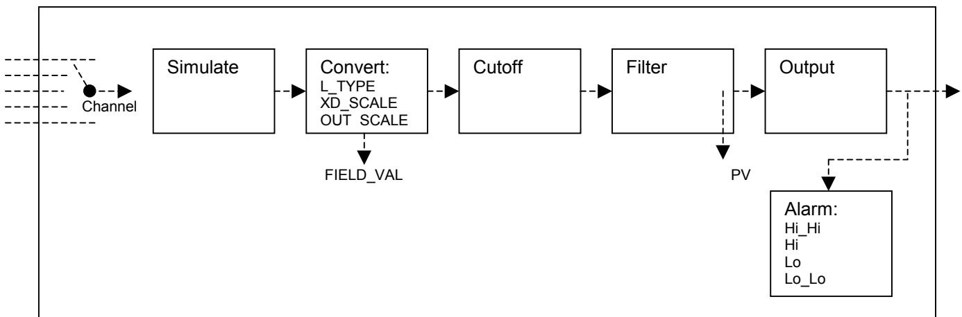
**Channel:** Using the channel parameter (index 15) you can choose the measured value to be transferred from the transducer block.
