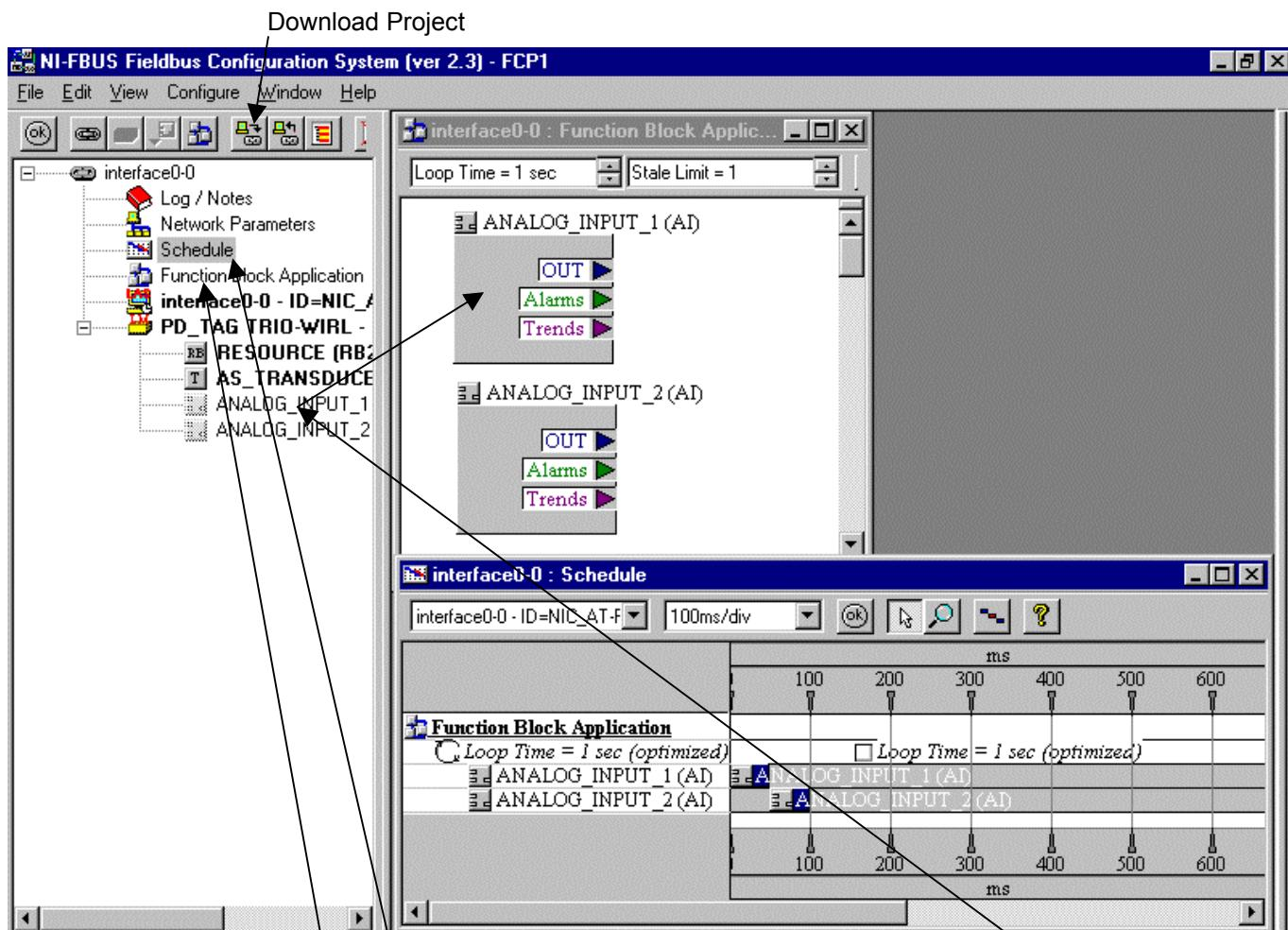
Please double-click on „Function Block Application“ to open this window. Then click on “Analog\_Input\_1” using the left mouse button. Keep the mouse button down. Drag the AI 1 symbol in the “Function Block Application” window. Should you want to make likewise use of AI2, repeat the above-mentioned procedure.
