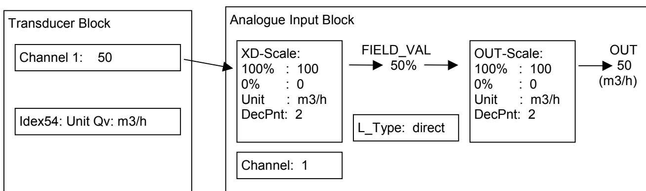
Using automatic operation mode the channel 1 value (see above example: "50") will automatically transferred through the AI block and then be displayed as OUT value "50".
