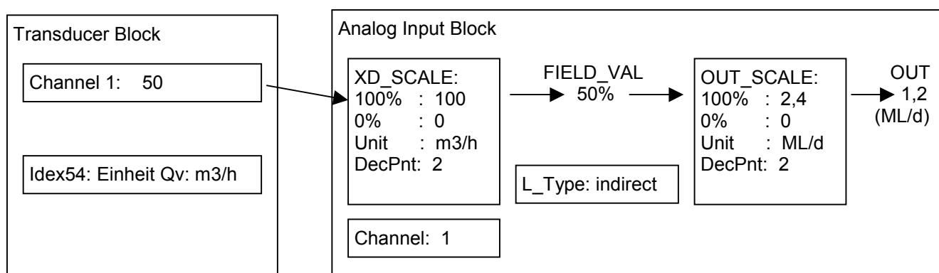
Using the XD scaling, the channel 1 value („50“ in this example) will then be automatically set to 50(%).
