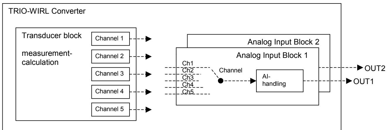
An AI block fulfils different tasks, such as change of scaling, alarm handling, simulation etc. See the following description:
