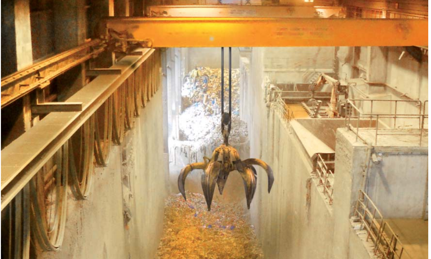
Using anti-sway control within the narrow bunker reduces collision damage.
