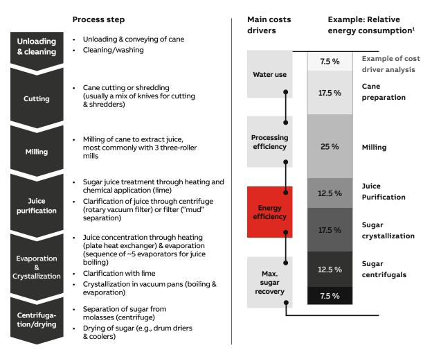
02 Sugarcane processing: main cost drivers and relative energy consumption of individual process steps
