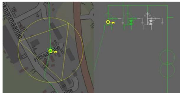
Figure 2. Remotely controlled CSS with fault indication in a DMS system
