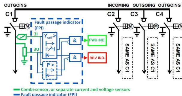
Figure 3. The principal concept of FPIs in compensated MV-networks
