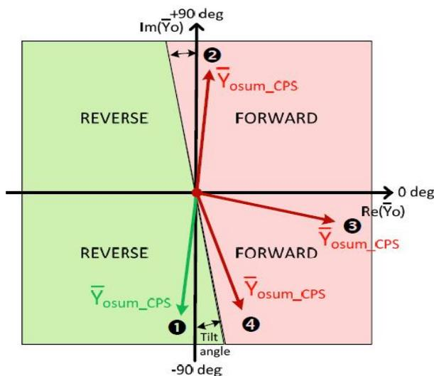
Figure 5. Illustration of the operation characteristics of the MFA-function
