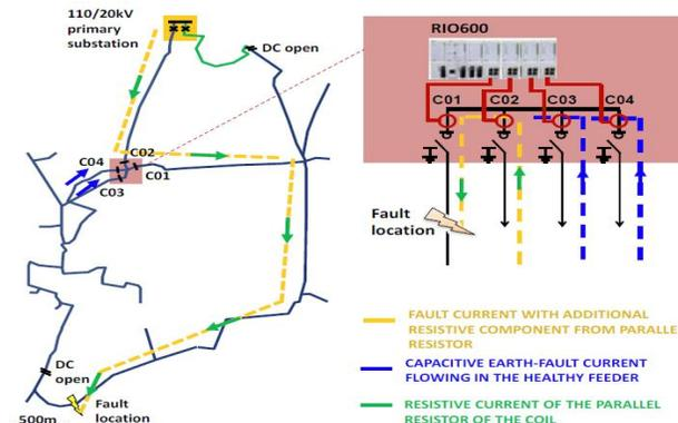
Figure 4. Fault currents flow paths in compensated MV-networks
