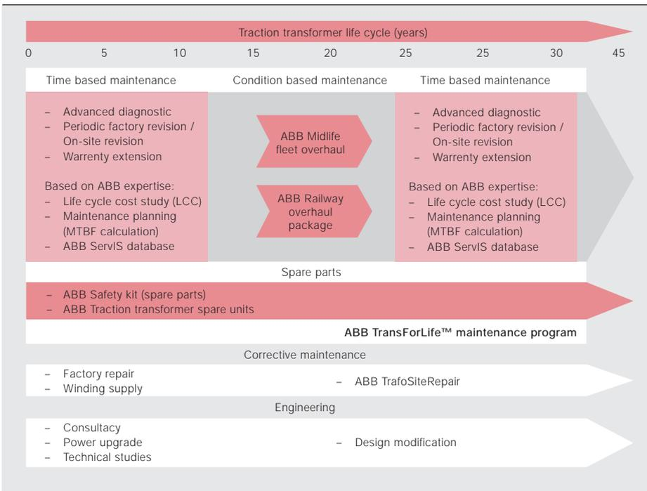
The company can draw on its broader knowledge by extending such offerings as parts of its ABB TransForLife™ solutions package to on-board traction transformers. This covers both on-site and factory repair/revision as well as maintenance contracts and spare parts. Similarly, traction transformers benefit from the company's simulation and diagnostics packages<sup>1</sup>.
