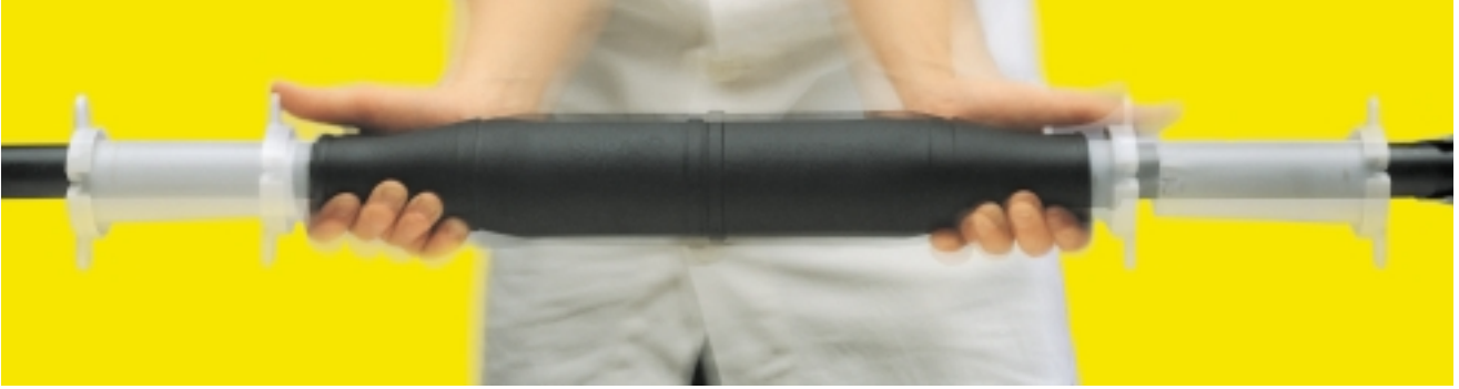
Fitting the SlipOver joint. After the conductors have been crimped together and the conducting cable layer removed, the fitter positions the joint, extracting the tensioning sleeves with a simple twisting movement. The joint collapses and fits snugly over the cable. 1
