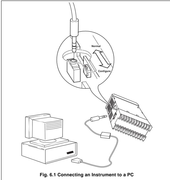
**Fig. 6.1 Connecting an Instrument to a PC**
