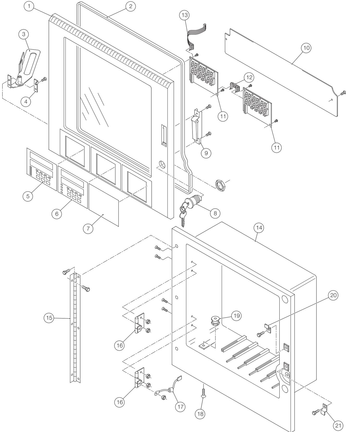
Figure 1 Replacement parts list – case components
