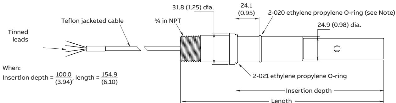
Note. 2-020 ethylene propylene O-ring location is not applicable to 100 mm (3.94 in) body length for 0.01 cell constant.
