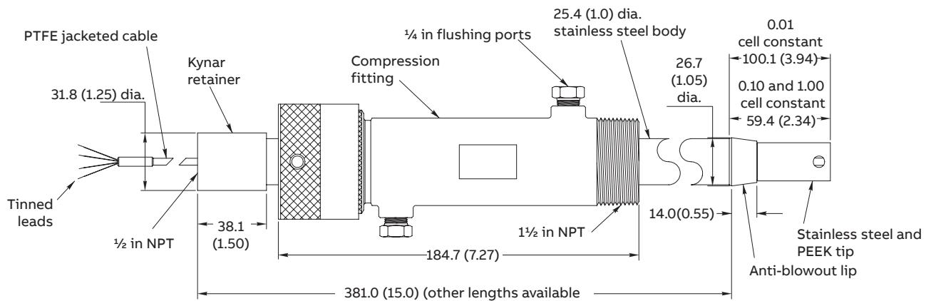
Hot tap with hand-tight flush and drain compression fitting
