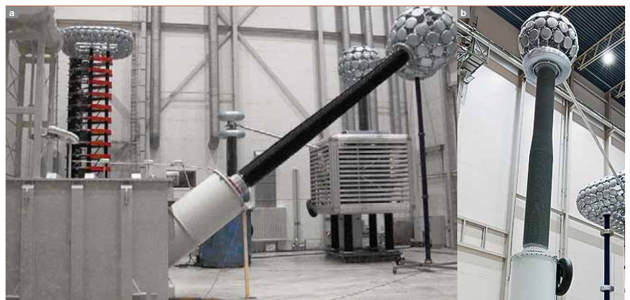
5 Extensive equipment testing is required before commercial 800kV HVDC can be offered commercially. These pictures show the transformer a , the transformer bushing b and the valve hall bushing (title photo, page 22) being tested in Ludvika, Sweden.
